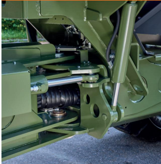
Without the need for a central drive shaft we can optimize the steering angle to 50° which generates an agile/nimble and low impact machine concept.
