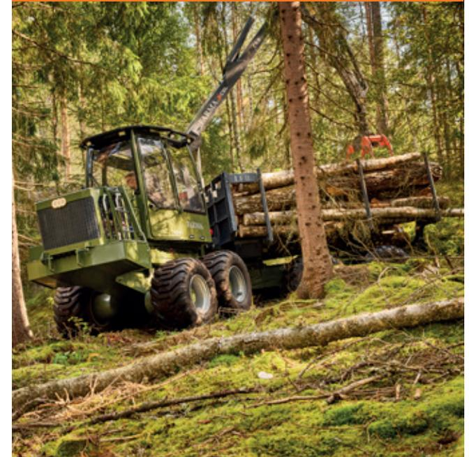
Optimized wheel speed, with full 8-wheel drive in forest work mode, results in less ground damage and less wear and tear on construction and transmission.
