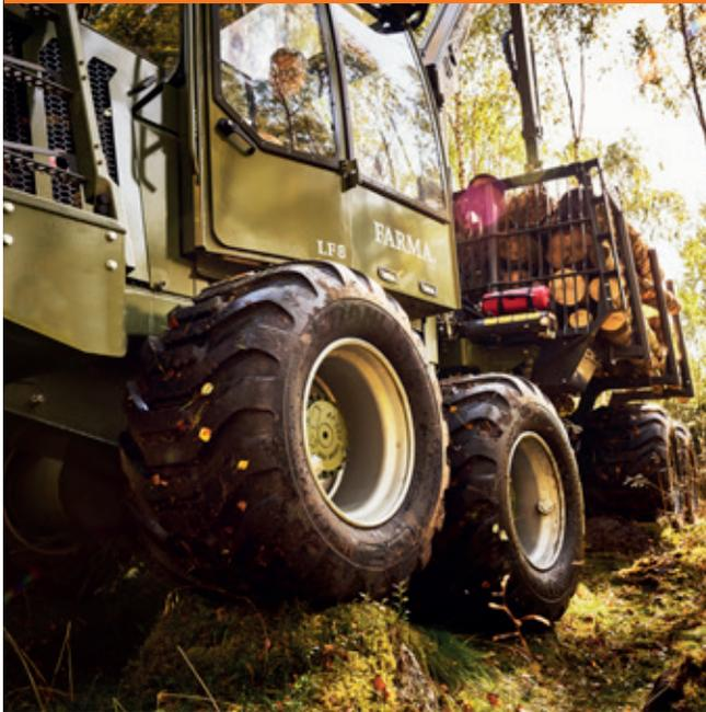
As the bogie axle is designed for wheel motors there is no rotating force transferred through the bogie axle bearing which can cause bogie lift/balancing issues or impair driver comfort. The Bogie axle is completely free to rotate and follow the terrain with optimal weight distribution and traction. Wheel motors guarantee full traction and climbing ability in all situations.
